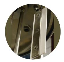
Outside sweeping blade is mounted with side scrapers at different levels to ensure materials are fed to the center. This allows for better heat transfer and keeps a consistent temperature throughout the product.
