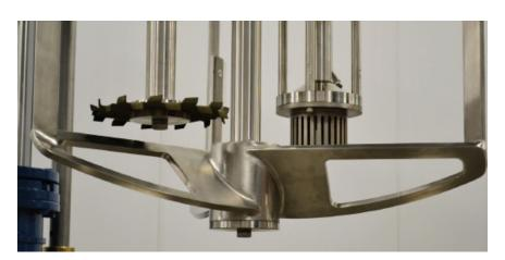
High speed disperser blade mounted to one shaft, rotor/ stator blade secured with rods for support on a second shaft and low speed sweeping blade. With the SMART package you can program and set independent start, stop and speed of each mixing blade.
